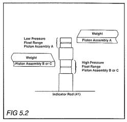
**Note:** Where variations of 0.0094 psi/0.00065 bar for Piston Assembly A (See Page 5) or 0.016 psi/0.0011 bar for Piston Assemblies B or C (See Page 5) are acceptable, then the bottom face of the lowest weight can align anywhere within the recessed area on the Indicator Rod.
