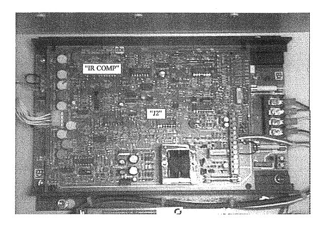
The "IR Comp" is used to stabilize motor speed under varying loads. When properly adjusted, the control will compensate so minimal motor speed change will occur over a wide range of motor loads.
